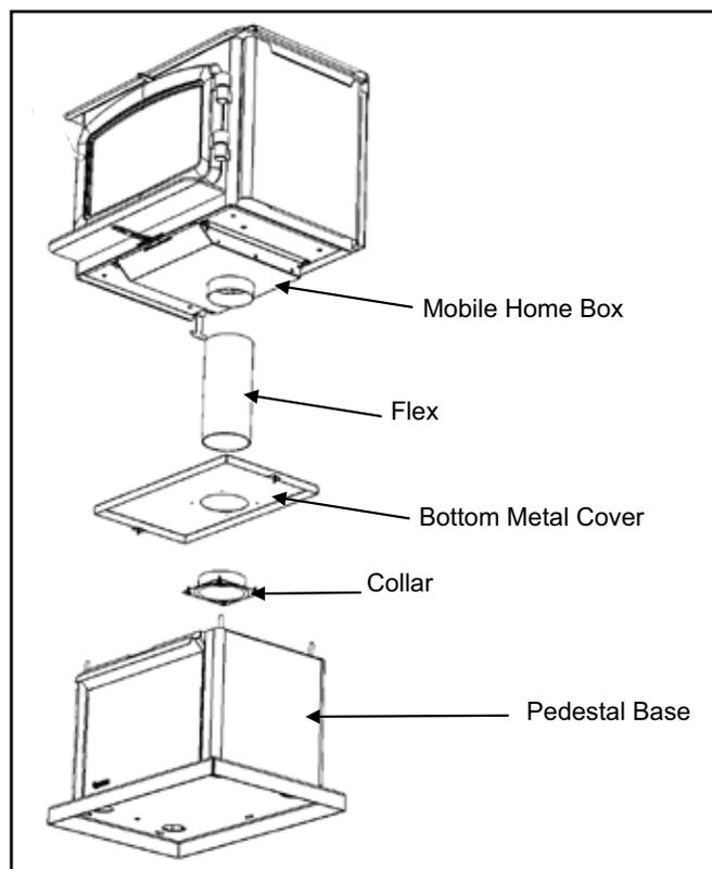
10. Secure collar to base of unit with 4 screws.
