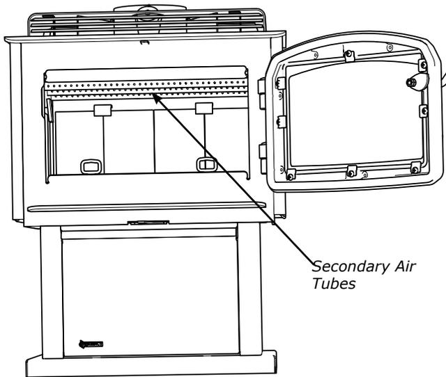
3. Grasp front secondary air tube firmly with vise grips, using a hammer tap vise grips from right to left until air tube is released from grip. Remove. See diagram 1. Repeat step to remove second airtube from front.
