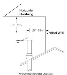
Figure 8 - Termination Cap clearances
