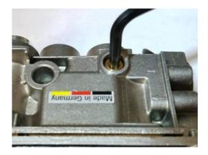
Figure 21 – Low Flow Orifice Removal
