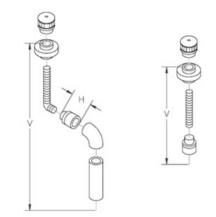
Figure 9 – Existing Chimney Venting Options
