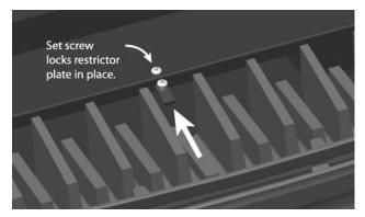
Figure 40 - Restrictor Fully Closed
