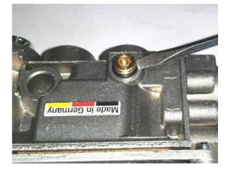
Figure 22 – Low Flow Orifice Removal – O-ring
