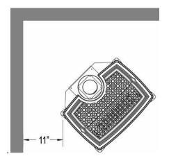
Figure 7 - Horizontal Vent Mantle Clearance
