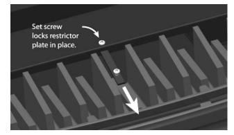
Figure 41 - Restrictor Fully Opened (no restriction)
