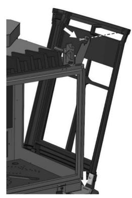
Figure 44 – Side Panel Mounting Detail
