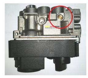
Figure 20 – Low Flow Orifice Location
