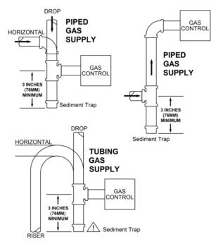
Figure 14 – Sample Gas Supply Sediment Traps
