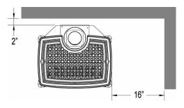
Figure 5 - Minimum Wall Clearances
