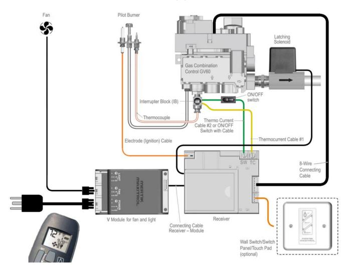
Figure 13 – Waitsfield 8770 Wiring Diagram
