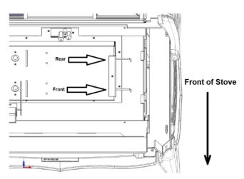
Figure 38 – Stove Bottom View: Air Shutter Adjusting Rods
