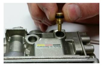
Figure 23 – NG Low Flow Screw Removal
